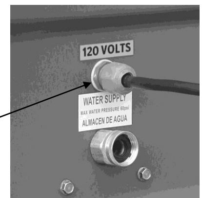
Electrical cord for 120V, 20Amp connection. Note: Standard 3/4" water connection for utility water source under 60 p.s.i.
