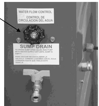
Top: Water control valve – controls water to units water reservoir. Open 1 ¼ turns. Bottom: Water hook-up for cleaning and flushing water reservoir.
